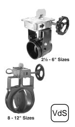
The Series 705W VdS butterfly valve features a weatherproof actuator housing approved for indoor or outdoor use. It has a ductile iron body and nickel plated disc with EPDM disc coating and nickel plated stem. The body is coated with a heat fused polyphenylene sulfide blend. The Series 705W VdS butterfly valve meets the VdS 2245 shutoff valve specifications and is approved for 16 Bar service.
