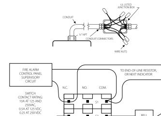
Switch 1: 2 leads per terminal Switch 2: 1 lead per terminal
