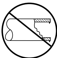
Unacceptable pipe end with burrs
