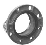
Style 994 HDPE flange adapter for HDPE pipe permits direct connection of ANSI Class 125 and 150 flanged components into HDPE systems. No fused adapters are required. The housing bolts onto the pipe end with sharp teeth to grip the pipe with tongue-and-groove for positive axial alignment. The Style 994 gasket seals on the pipe O.D. and directly to the flange face. No standard flange gasket is required.
