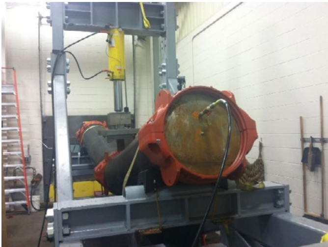
Figure 2. Flexure test being performed on 24" IPS Victaulic Style 908 coupling assemblies.
