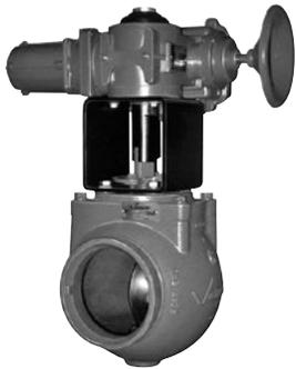
Plug valves are designed to accommodate a variety of remote actuators – electric, pneumatic, and hydraulic. The design featuring PTFE thrust washers, self-lubricating bearings and eccentric plug design, serves to reduce break-away torque requirements.
