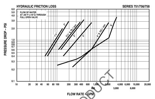
The chart below expresses the frictional resistance of Victaulic Series 756 Dry Check Valve in equivalent feet of straight pipe.
