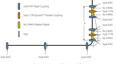
Example of Style 177N QuickVic<sup>™</sup> Flexible Coupling Deflection Capabilities
