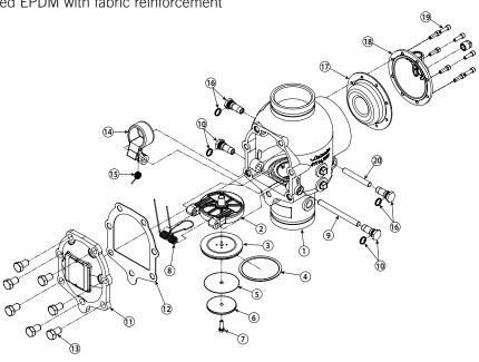
The  $1\frac{1}{2}$ "/DN40 and 2"/DN50 valve sizes contain washers under the heads of the cover plate bolts.
