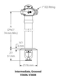
For wet system installation or dry/preaction systems installed in areas above 40°F/5°C
