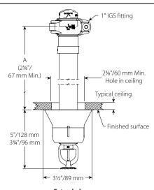
Extended Sleeve and Skirt, Grooved V3606, V3608
