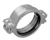
The new Aquamine® Style 2972 transition coupling provides the convenience of bolted, mechanical assembly for plain-end PVC pipe to grooved-end steel pipes, valves, and fittings. This coupling allows you to join shorter sections of PVC pipe, or insert fittings and valves into a pipe section without having to use special adapters.
