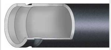
Roll groove profile (exaggerated for clarity). The small dimple created on interior pipe wall has minimal effect on pressure or flow.
