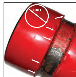
BAD PIPE END CONTAINS PUCKERED/ WAVY PAINT ON THE "A" DIMENSION
