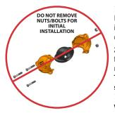
**1. DO NOT DISASSEMBLE THE FITTING FOR INITIAL INSTALLATION:** Victaulic<sup>®</sup> FireLock<sup>™</sup> No. 101 and 103 Installation-Ready<sup>™</sup> Fittings are designed so that the installer does not need to remove the nuts and bolts for initial installation. This facilitates installation by allowing the installer to directly insert the grooved end of mating components into the fitting.
