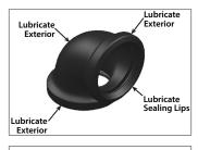
3a. VERIFY THAT THE CORRECT-SIZE GASKET IS BEING USED FOR REASSEMBLY.
