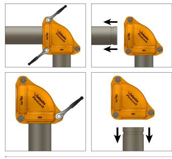
2. Loosen the nuts only on the outside and inside locations of the fitting end where the first mating component is to be removed (nuts should be threaded no further than flush with the end of the bolts). Remove the mating component from the loosened side. Verify that the fitting is secured to the other mating component to prevent the fitting from falling.
