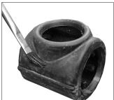
**2. LUBRICATE GASKET:** Apply a thin coat of a compatible lubricant to both of the gasket sealing lips and the entire gasket exterior. Refer to the "Lubricant Compatibility for Gaskets" table on page 2.
