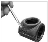
**5. FOR REASSEMBLY OF STYLE 118 OUTLET COUPLINGS, LUBRICATE GASKET:** Apply a thin coat of a compatible lubricant to both of the gasket sealing lips and the entire gasket exterior. Refer to the "Lubricant Compatibility for Gaskets" table on page 2.
