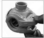
**3. INSTALL GASKET INTO OUTLET HOUSING**: Install the gasket into the outlet housing. Verify that the housing's outlet engages with the outlet portion of the gasket.
