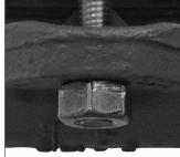
**4. INSTALL BOLT AND NUT:** Install the bolt into the outlet housing, as shown to the left, and thread a nut onto the bolt. **NOTE:** Verify that the oval neck of the bolt seats properly in the bolt hole. DO NOT tighten the nut completely. The bolt pads need to be set at a gap for reinstallation of the coupling. The nut should be flush with the top of the bolt to provide the proper gap.
