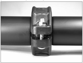
**4a.** Align and bring the two pipe/fitting ends together. Slide the coupling into position so that the coupling keys align with the groove in each pipe/fitting. A visual check is required to ensure the coupling keys align with the grooves in the pipe/fitting. **NOTE:** The coupling may be rotated to ensure the gasket is seated properly.
