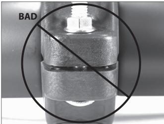
**6.** Visually inspect the bolt pads at each joint to ensure full bolt-pad to bolt-pad contact is achieved.
