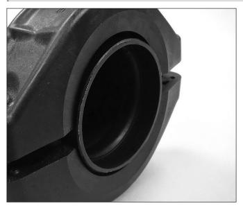
**4. INSTALL COUPLING OVER PIPE/FITTING END:** Position the coupling over the grooved pipe/fitting end. Make sure the coupling and gasket do not overhang the pipe/fitting end.
