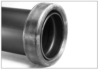
**3a. POSITION GASKET:** Position the gasket over the grooved pipe/ fitting end. Make sure the gasket does not overhang the pipe/fitting end.
