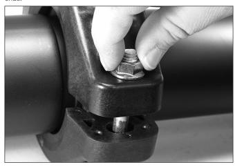
**6. INSTALL BOLTS/NUTS:** Install the bolts, and thread a nut fingertight onto each bolt. **NOTE:** Make sure the oval neck of each bolt seats properly in the bolt hole.
