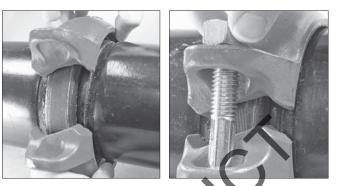
**7. INSTALL HOUSINGS:** Install the housings over the gasket. Make sure the housings' keys engage the grooves properly on both pipes/mating components.
