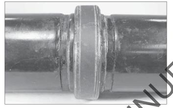
**5. JOIN PIPE/MATING COMPONENTS:** Align the two grooved ends of the pipe/mating components. Insert the other pipe/mating component end into the gasket until it contacts the center leg of the gasket. **NOTE:** Make sure no portion of the gasket extends into the groove of either pipe/mating component.
