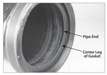
**4. INSTALL GASKET:** Insert the grooved end of a pipe/mating component into the gasket until it contacts the center leg of the gasket.
