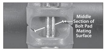
**NOTE:** It is possible to bring the outside sections of the bolt pads into metal-to-metal contact without having metal-to-metal contact at the middle section of the bolt pad mating surfaces. Tightening the nuts evenly by alternating sides is required to bring the entire bolt pad sections into metal-to-metal contact. Refer to the graphics on the following page for details.
