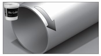
1. Make sure the interior surface of the coupling body is clean. Apply an even coat of lubricant (provided with the product) to the interior surface of the coupling body, both sides of the sealing plate, and both pipe ends (total width of a coupling body back from the pipe ends), as shown.
