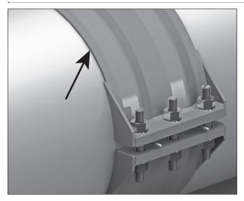
**10.** Proper assembly is achieved when the coupling body is in full contact with the pipe surface. However, a gap between the coupling body/shoulders and the pipe is acceptable if it does not exceed the following specifications.
