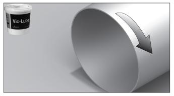
1. Make sure the interior surfaces of the coupling bodies are clean. Apply an even coat of lubricant (provided with the product) to the interior surfaces of each coupling body, both sections of the coupling bodies that will slide underneath each other, both sides of the sealing plates, and both pipe ends (total width of a coupling body back from the pipe ends), as shown. NOTE: Use of reference marks on the pipe is recommended.
