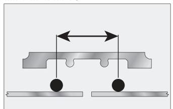
**3.** Measure the center-to-center distance between the o-ring pockets. Position the center of the o-rings this measured distance apart around the entire pipe circumference. Keep the pipe gap centered between the o-rings.
