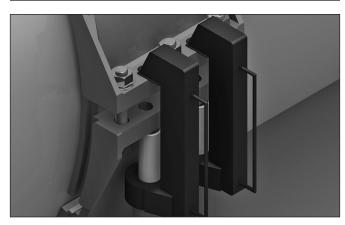
**8.** Slowly begin to close the coupling bodies with the closure tools, while making sure the sealing plates slide between the coupling bodies and the o-rings without bending or tearing.
