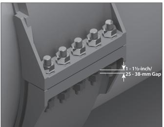
**6a.** Allow the closure plates on one side to contact. Apply lubricant (provided with the product) to the threads of all carbon steel studs. **NOTE:** Anti-seize lubricant is required for stainless steel fasteners. Insert studs with flat washers into the holes. Apply nuts loose enough to allow a  $1 - 1\frac{1}{2}$ -inch/25 - 38-mm gap between the closure plate and nuts, as shown above.
