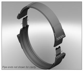
**6.** Position the other coupling body over the pipe joint with the o-rings seated in the o-ring pockets. Make sure the o-rings do not shift out of position. **NOTE:** The graphic above shows the upper and lower bodies and their relation with the sealing plates. Make sure the extended body section of the coupling is placed between the sealing plate and the overlapping reinforcement so that the sealing plate is seated between the coupling body and the o-rings.
