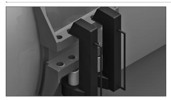
**7.** On the opposite side of the coupling bodies, place the pin of each closure tool head into the two inside holes of the closure plate, as shown above. Place the pin on the end of the hydraulic rams into the corresponding holes of the other closure plate.
