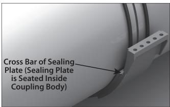
**5.** Insert a sealing plate, with the cross bar facing out, between the coupling body and o-rings on each side of the coupling body, as shown above.
