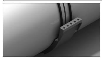
**4.** When possible, center one coupling body below the pipe joint. Raise the bottom coupling body until it contacts the o-rings installed on the pipe. Make sure the o-rings are seated in the o-ring pockets and that they do not shift out of position. When the bottom coupling body is positioned properly, use cribbing to stabilize and maintain this position. **NOTE:** Depending on field conditions, the upper coupling body can be installed first.
