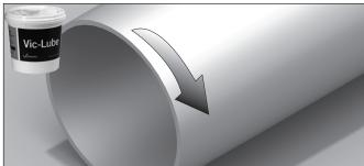
**2.** Make sure the interior surface of the coupling body is clean. Apply an even coat of lubricant (provided with the product) to the interior surface of the coupling body, both sides of the sealing plate, and both pipe ends (total width of a coupling body back from the pipe ends), as shown.
