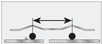
**5.** Measure the center-to-center distance between the arches. Position the center of the o-rings this measured distance apart around the entire pipe circumference, as shown above.
