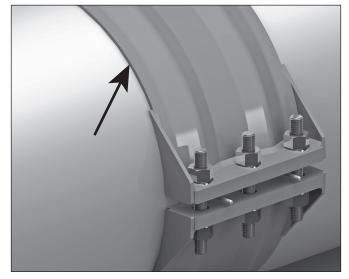
11. Proper assembly is achieved when the coupling body is in full contact with the pipe surface around the circumference of the pipe. However, a gap between the coupling body and the pipe is acceptable if it does not exceed  $\frac{1}{16}$  inch/1.6 mm and totals no more than 10% of the pipe circumference.
