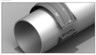
**3.** Slide the lubricated coupling body over one of the pipe ends.
