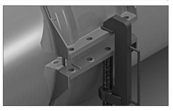
**7.** When an even number of closure plate holes exists, place the pin of the closure tool head into the center hole closer to the steel shoulder of the coupling body. Place the pin on the end of the hydraulic ram into the corresponding center hole of the other closure plate.
