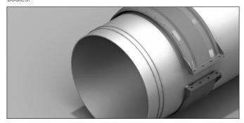
3. Slide the lubricated coupling body over one of the pipe ends, as shown above. The side of the coupling body that contains the Teflon\* shoulder must be installed toward the pipe end that contains the cladding.
