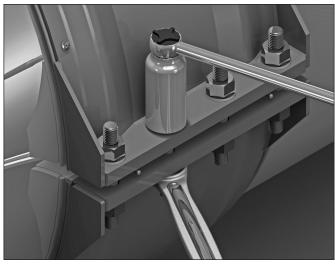
10. Finish closing the coupling body by tightening the fasteners gradually and evenly until the coupling body is in full contact with the pipe around its circumference. The closure plates should not contact each other.
