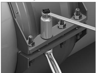
10. Finish closing the coupling body by tightening the fasteners gradually and evenly until the coupling body is in full contact with the pipe around its circumference. The closure plates should not contact each other.
