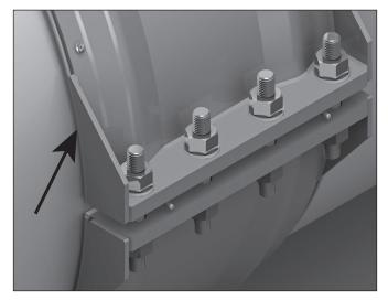
11. Proper assembly is achieved when the coupling body is in full contact with the pipe surface around the circumference of the pipe. However, a gap between the shoulder and the pipe is acceptable if it does not exceed 3/32 inch/2.4 mm and totals no more than 10% of the pipe circumference.
