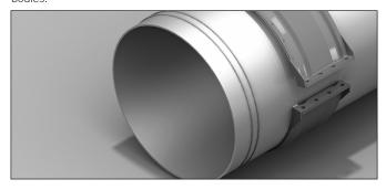
3. Slide the lubricated coupling body over one of the pipe ends. The side of the coupling body that contains the Teflon\* shoulder must be installed toward the pipe end that does not contain restraint rings.
