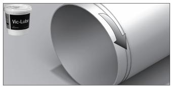
**2.** Make sure the interior surface of the coupling body is clean. Apply an even coat of lubricant (provided with the product) to the interior surface of the coupling body, both sides of the sealing plate, and both pipe ends (total width of a coupling body back from the pipe ends), as shown.
