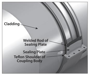
**6.** Insert a sealing plate, **with the pins facing out**, between the coupling body and o-rings on each side of the coupling body, as shown above. **NOTE:** The Teflon spacer on the sealing plates must be installed toward the Teflon shoulder of the coupling bodies.
