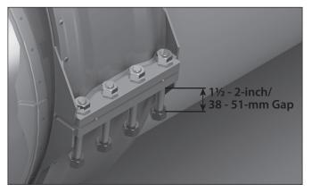
7. Position the other coupling body over the pipe joint with the o-rings seated in the arches. The side of the coupling body that contains the Teflon shoulder must be installed toward the pipe end that contains the cladding. Make sure the o-rings do not shift out of position.
