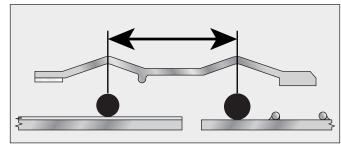
**4.** Measure the center-to-center distance between the arches. Position the center of the o-rings this measured distance apart around the entire pipe circumference, as shown above.
