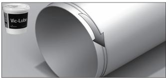
2. Make sure the interior surfaces of the coupling bodies are clean. Apply an even coat of lubricant (provided with the product) to the interior surfaces of each coupling body, both sides of the sealing plates, and both pipe ends (total width of a coupling body back from the pipe ends), as shown.
