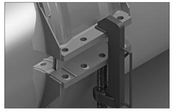
**8.** On the opposite side of the coupling bodies: When an even number of closure plate holes exists, place the pin of the closure tool head into the center hole closer to the steel shoulder of the coupling bodies. Place the pin on the end of the hydraulic ram into the corresponding center hole of the other closure plate.
