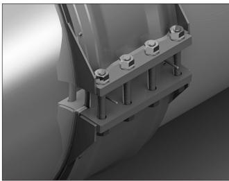
10. Remove the closure tool and insert a stud with flat washers and nuts into each of the remaining hole(s).
