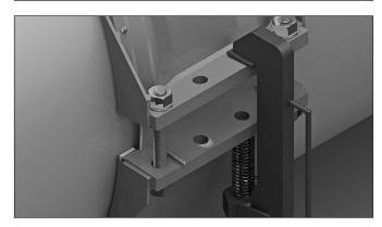
**9.** Slowly begin to close the coupling bodies with the closure tool, while making sure the sealing plates slide between the coupling bodies and the o-rings without bending or tearing.
