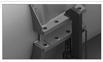
8. On the opposite side of the coupling bodies: When an even number of closure plate holes exists, place the pin of the closure tool head into the center hole closer to the steel shoulder of the coupling bodies. Place the pin on the end of the threaded rod or the hydraulic ram into the corresponding center hole of the other closure plate.
