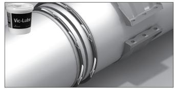
**4.** Slide one o-ring over each lubricated pipe end. The o-rings are designed to fit tight and will require stretching to fit around the pipe diameter. Apply lubricant to the o-rings after they are placed on the pipe ends by lifting the o-rings and applying lubricant around the diameter. Place the bonded area of the o-rings away from the opening of the coupling body that is intended for the sealing plate location. Make sure all twists are removed from the o-rings.
