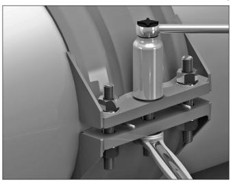
**10.** Finish closing the coupling body by tightening the fasteners gradually and evenly until the coupling body is in full contact with the restraint rings and pipe around its circumference. The closure plates should not contact each other.
