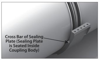
**6.** Insert a sealing plate, with the cross bar facing out, between the coupling body and o-rings on each side of the coupling body, as shown above
