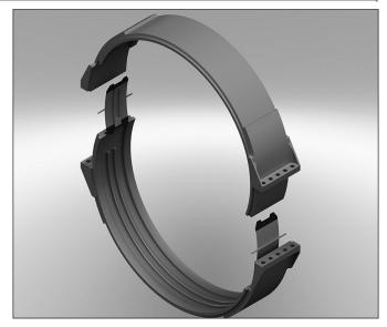
**7.** Position the other coupling body over the pipe joint with the o-rings seated in the o-ring pockets. Make sure the o-rings do not shift out of position. **NOTE:** The graphic above shows the upper and lower bodies and their relation with the sealing plates. Make sure the extended body section of the coupling is placed between the sealing plate and the overlapping reinforcement so that the sealing plate is seated between the coupling body and the o-rings.
