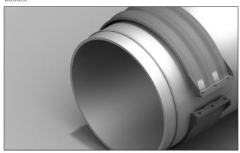
**3.** Slide the lubricated coupling body over one of the pipe ends beyond the restraint ring.
