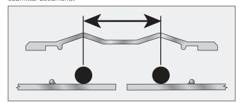
**5.** Measure the center-to-center distance between the arches. Position the center of the o-rings this measured distance apart around the entire pipe circumference. Keep the pipe gap centered between the o-rings.
