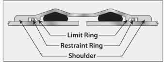
**5a.** The restraint rings must be located between the shoulders and limit rings.
