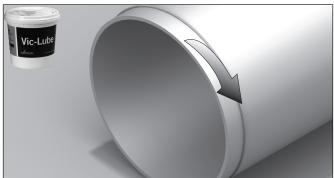
**2.** Make sure the interior surface of the coupling body is clean. Apply an even coat of lubricant (provided with the product) to the interior surface of the coupling body, both sides of the sealing plate, and both pipe ends (total width of a coupling body back from the pipe ends), as shown.
