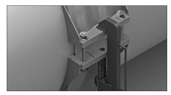
**9.** Slowly begin to close the coupling bodies with the closure tool, while making sure the sealing plates slide between the coupling bodies and the o-rings without bending or tearing. Make sure the shoulders are closing on the outside of the restraing rings.
