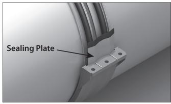
**6.** Insert a sealing plate, **with the pins facing out**, between the coupling body and o-rings on each side of the coupling body, as shown above.
