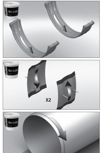
**2.** Make sure the interior surfaces of the coupling bodies are clean. Apply an even coat of lubricant (provided with the product) to the interior surfaces of each coupling body, both sides of the sealing plates, and both pipe ends (total width of a coupling body back from the pipe ends), as shown.
