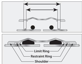
**4a.** The restraint rings must be located between the shoulders and limit rings.
