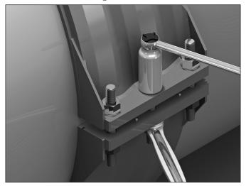
**11.** Finish closing the coupling bodies by tightening each set of hardware gradually, alternating between the two closure plate locations, until the coupling bodies are in full contact with the pipe around its circumference. The closure plates should not contact each other.
