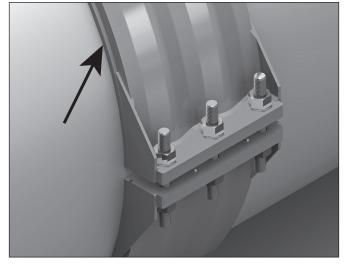
**12.** Proper assembly is achieved when the coupling bodies are in full contact with the pipe surface. However, a gap between the shoulder and the pipe is acceptable if it does not exceed  $\frac{3}{22}$  inch/2.4 mm and totals no more than 10% of the pipe circumference
