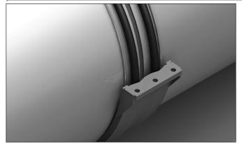
**5.** When possible, center one coupling body below the pipe joint. Raise the bottom coupling body until it contacts the o-rings installed on the pipe. Make sure the o-rings are seated in the arches and that they do not shift out of position. When the bottom coupling body is positioned properly, use cribbing to stabilize and maintain this position. **NOTE:** Depending on field conditions, the upper coupling body can be installed first.
