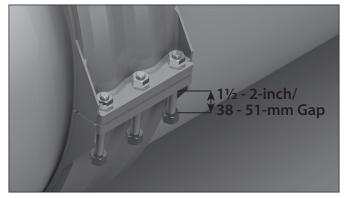
**7.** Position the other coupling body over the pipe joint with the o-rings seated in the arches. Make sure the o-rings do not shift out of position.
