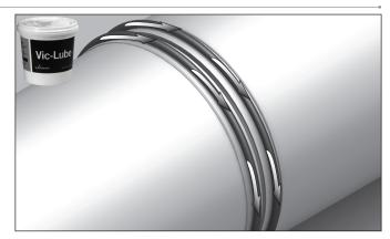
**3.** Slide one o-ring over each lubricated pipe end. The o-rings are designed to fit tight and will require stretching to fit around the pipe diameter. Apply lubricant to the o-rings after they are placed on the pipe ends by lifting the o-rings and applying lubricant around the diameter. Place the bonded area of the o-rings away from the openings of the coupling bodies that are intended for the sealing plate locations. Make sure all twists are removed from the o-rings.
