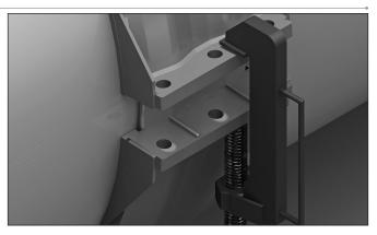
**8.** On the opposite side of the coupling bodies, place the pin of the closure tool head into one of the center holes of the closure plate, as shown above. Place the pin on the end of the threaded rod or the hydraulic ram into the corresponding center hole of the other closure plate.
