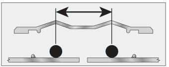
**4.** Measure the center-to-center distance between the arches. Position the center of the o-rings this measured distance apart around the entire pipe circumference. Keep the pipe gap centered between the o-rings. Make sure the o-rings are not twisted.
