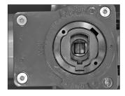
3. Verify that the valve is in the fully "shut" position. The fully "shut" position can be verified by removing the indicator cap from the top of the gear operator and checking the position indicator on top of the stem, as shown to the left. The position indicator line on top of the stem should be in-line with the "shut" position.
