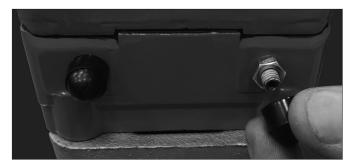
1. Remove the dust cap from the right side of the gear operator.
