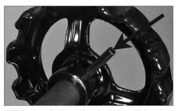
**NOTE:** For 10-inch/DN250 and 12-inch/DN300 Series 250 Butterfly Valves, the handwheel is not attached to the shaft. To attach the handwheel to the shaft, align the holes in the handwheel with the holes in the shaft. Drive the roll pin (provided/taped to handwheel) completely into the handwheel and shaft.
