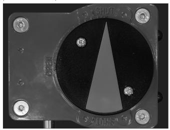
2. Turn the handwheel of the gear operator until the arrow on the indicator cap is pointing toward the "shut" position, as shown above.
