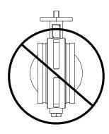
DO NOT INSTALL BUTTERFLY VALVES INTO THE SYSTEM WITH THE DISC IN THE FULLY-OPEN POSITION. Exposed disc may be damaged and prevent proper function of the valve.
