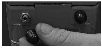
1. Remove the dust cap from the left side of the gear operator.
