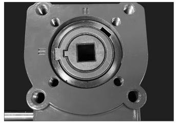
3. Insert the drive bushing into the gear operator, as shown above.
