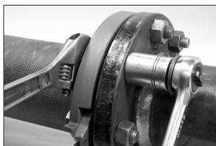
4-Bolt Tightening Pattern
