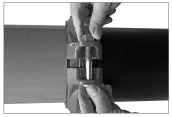
**4. INSTALL HOUSINGS:** Install the housings over the gasket. Verify that the sides of the two housings marked "CPVC/PVC" are facing the CPVC/ PVC pipe and that the housings' keys engage the grooves completely on both mating components.
