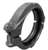
• METHOD 1 FOR REASSEMBLY: The coupling can be reassembled into its "installation-ready" condition by installing the gasket into the housings, then inserting the bolts and threading a nut onto each bolt until 2 – 3 threads are exposed, as shown above. Verify that the sides of the two housings marked "CPVC/PVC" are facing the same direction. If this method is chosen, steps 1 – 3 in the left column, along with all steps on page 2, shall be followed.
