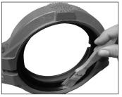
4. LUBRICATE GASKET: Apply a thin coat of Victaulic Lubricant only to the sealing lips of the gasket. NOTE: The gasket exterior is supplied with a factory-applied lubricant, so it is not necessary to remove the gasket from the housings to apply additional lubricant to the exterior surface.
