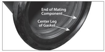
**2. INSTALL GASKET:** Insert the grooved end of a mating component into the gasket until it contacts the center leg of the gasket.
