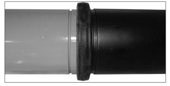
**3. JOIN MATING COMPONENTS:** Align the two grooved mating component ends. Insert the other mating component end into the gasket until it contacts the center leg of the gasket. **NOTE:** Verify that no portion of the gasket extends into the groove of either mating component.
