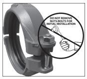
1. DO NOT DISASSEMBLE THE COUPLING: Style 356 Installation-Ready<sup>™</sup> Transition Couplings are designed so that the installer does not need to remove the bolts and nuts for installation. This design facilitates installation by allowing the installer to directly insert the grooved end of mating components into the coupling.
