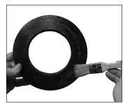
2. CHECK GASKET AND LUBRICATE: Check the gasket to verify that it is suitable for the intended service. The color code identifies the material grade. Refer to Victaulic publication 05.01 for the color code chart, which can be downloaded at victaulic. com. Apply a thin coat of Victaulic Lubricant to the gasket sealing lips and exterior.
