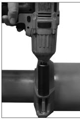
7. TIGHTEN NUTS: Tighten nuts evenly by alternating sides until metalto-metal contact occurs at the bolt pads. Verify that the oval neck of each bolt seats properly in the bolt hole and that housings' keys engage the grooves completely on both mating components.
