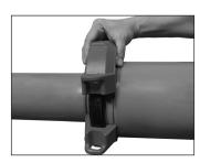
**5. INSTALL HOUSINGS:** Install the housings over the gasket. Verify that the larger openings of the housings are facing the larger mating component and that the housings' keys engage the grooves completely on both mating components.
