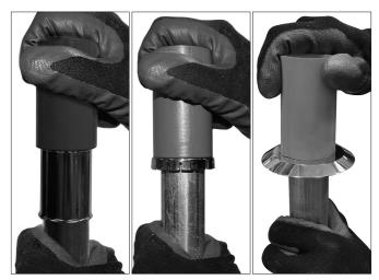
**3.** Using the tool provided, push down on the sleeve, recessed collar, or flush plate just until it is retained in the groove of the barrel. Use caution when using this tool to prevent damage to the bulb, deflector, and frame arms
