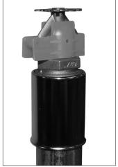
4. Reinstall the bulb protector onto the sprinkler to protect the bulb during sprinkler installation. Use caution when reinstalling the bulb protector to prevent damage to the bulb, deflector, and frame arms. DO NOT use any tools to reinstall the bulb protector. Sprinklers showing any signs of damage shall be replaced immediately.
