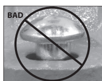
OVAL NECK OF BOLT NOT SEATED PROPERLY
