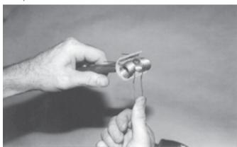
Grasp the tongue of the torsion spring with one hand and the handle of the tool with the other hand. Wind the tongue 180° until it contacts the edge of the guide.
