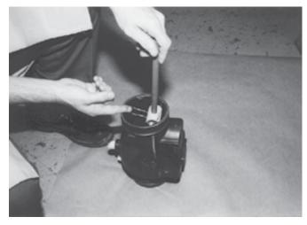
7. Insert the torsion spring and tool into the valve body. Position the coils between the ears of the disc in alignment with the shaft holes. White continuing to hold the tool, release the tongue of the torsion spring so that it presses against the center of the disc without unwinding.
