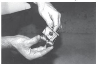
5. Insert the arms of the torsion spring (provided in the kit) into the holes at the edges of the curved guide of the installation tool (Item 7 provided in the kit). The coils of the torsion spring should be seated fully against the guide and on opposite sides of the center spacer.
