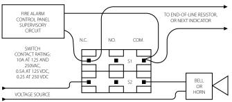
Switch 1: 2 leads per termina Switch 2: 1 lead per terminal
