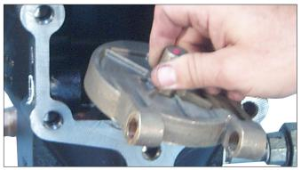
Remove the clapper assembly from the valve body seat ring. Clean out any holes that are plugged in the valve body seat ring. DO NOT USE SOLVENTS OR ABRASIVES.
