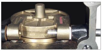
Start the clapper shaft into the valve body and place one spacer between the clapper and valve body, as shown above.
