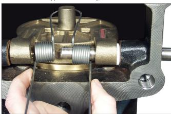
Install the clapper spring onto the clapper shaft. Verify that the loop of the clapper spring is facing the clapper, as shown above.
