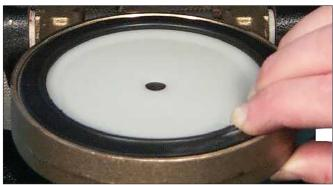
Install the clapper seal into the clapper carefully.
