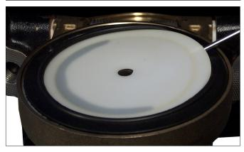
Pry the edge of the old seal washer from inside the clapper seal, as shown above.
