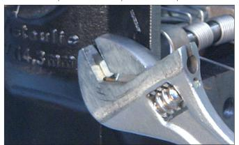
2. Remove the clapper shaft retaining plugs from the valve body.
