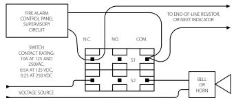
Switch 1: 2 leads per terminal Switch 2: 1 lead per terminal
