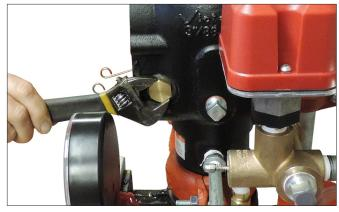
**2.** Remove the clapper shaft bushings with o-rings from the valve body.
