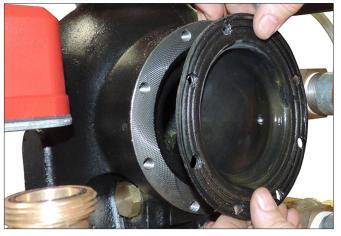
**4.** Remove the diaphragm from the valve body. Discard the diaphragm.
