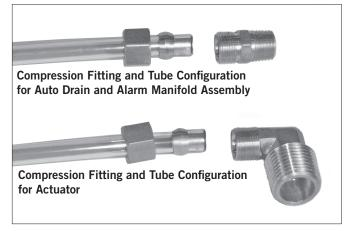
Compression fittings and tubes are provided for connection from the outlet of the auto drain, alarm manifold assembly, and actuator to the drip cup or drain. Install the compression fittings in accordance with the trim drawing provided. NEVER INSERT A PLUG INTO THE OUTLET OF THE AUTO DRAIN, ALARM MANIFOLD ASSEMBLY, OR ACTUATOR IN PLACE OF THE COMPRESSION FITTING/TUBE.
