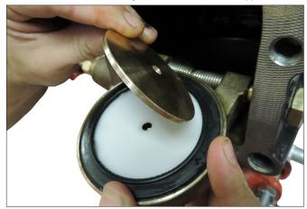
**3.** Remove the seal-retaining ring. Save the seal-retaining ring for re-installation.
