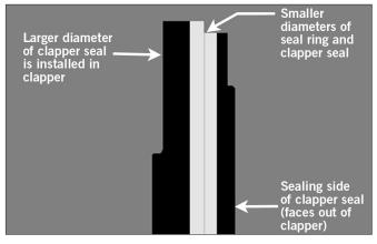
**6a.** If using the same clapper seal assembly and the seal ring was removed from the clapper seal in the previous step: Re-insert the seal ring carefully underneath the outer lip of the clapper seal. Ensure that the smaller diameter of the seal ring is toward the sealing surface of the clapper seal.
