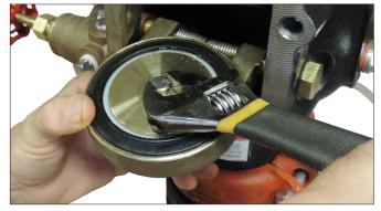
2. Remove the seal assembly bolt/bolt seal from the clapper seal.
