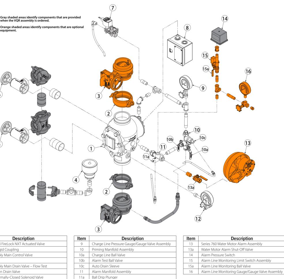
**2.** Open the water supply main drain valve (Item 5) fully to flush the water supply of any contaminants.
