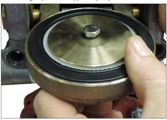
Place the seal-retaining ring onto the seal washer of the clapper seal. Install the seal assembly bolt/bolt seal through the sealretaining ring and clapper.
