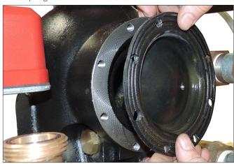
Remove the diaphragm from the valve body. Discard the diaphragm.
