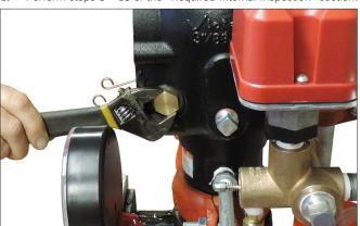
Remove the clapper shaft bushings with o-rings from the valve body.
