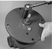
**6.** Reinstall and tighten the two mounting bolts.
