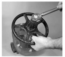
**2** Reinstall and tighten the operator retaining nut. To prevent the valve shaft from turning, restrain the handwheel.
