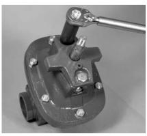
**2** Loosen and remove the two stem seal flange mounting bolts from the valve.
