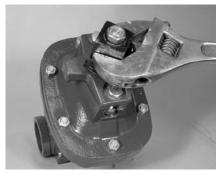
**1.** Fully open the valve by turning the square operating nut counterclockwise until you feel a sharp resistance.
