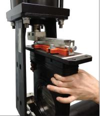
7. REMOVE CARTRIDGE: When the seat has cleared the opening of the valve body, slide the seat cartridge out from the slot in the gate connector.
