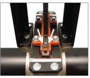
9. INSPECT GAP: Operate the handwheel (or the pneumatic or hydraulic operator) to raise the knife out of the valve body. Ensure that the gap on both sides of the knife is equal. The hex cap screws of the packing gland can be adjusted, if necessary, to achieve an equal gap on both sides of the knife. Refer to the Installation and Maintenance Instructions for details.
