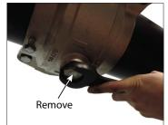
**3. REMOVE PLUG:** Using a 1½-inch/32 mm wrench (for the 3 to 8" valves) or a 1½-inch/38 mm wrench (for the 10 to 12" valves), remove the plug from the bottom of the valve body
