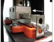
INSERT CARTRIDGE: Slide the replacement seat cartridge into the slot in the gate connector.
