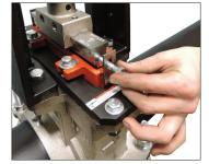
**4. REMOVE AND RELOCATE GATE CONNECTOR SCREWS:** Remove the two hex cap screws from the gate connector. Relocate them through the tab on each side of the seat and into the side of the knife, then finger-tighten. This is necessary to attach the seat to the knife during removal in later steps.
