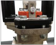
**3b.** For pneumatically and hydraulically operated valves, actuate the valve closed to bring the seat toward the valve body.
