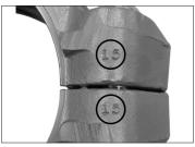
6. MATCH HOUSINGS: The housings are marked with a number/letter combination on each bolt pad. During installation, the housings' bolt pads shall be mated so that the same number/letter combination is matched.
