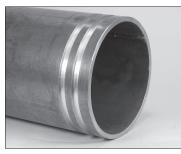
1. CHECK PIPE ENDS: The outside surface of the pipe, between the groove and the pipe ends, shall be generally free from indentations, projections, weld seam anomalies, and roll marks to ensure a leak-tight seal. All oil, grease, loose paint, dirt, and cutting particles shall be removed.
