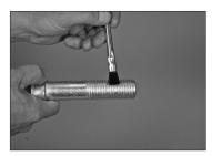
8. LUBRICATE BOLT THREADS: Lubricate the bolt threads with a thin coat of compatible lubricant.
