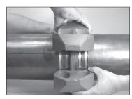
7. INSTALL HOUSINGS: Install the housings over the gasket. Verify that the housings' keys engage each groove completely on both pipe ends.
