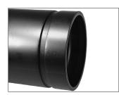
2. CHECK MATING COMPONENT ENDS: The outside surface of the mating components, between the groove and the mating component ends, shall be generally free from indentations, projections, weld seam anomalies, and roll marks to ensure a leak-tight seal. All oil, grease, loose paint, dirt, and cutting particles shall be removed.
