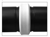
5. JOIN MATING COMPONENTS: Align and bring the two mating component ends together. Slide the seal assembly into position by centering it between the groove in each mating component end. NOTE: Verify that no portion of the seal assembly extends into the groove of either mating component.
