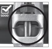
10. INSPECT BOLT PADS: Inspect the bolt pads at each joint to verify that proper assembly is achieved. The nuts shall be torqued to the values listed in the table below. In addition, the gap at each set of bolt pads shall be relatively even (the sum of the gap at both bolt pad locations shall not exceed the dimension listed in the table below).
