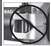
NO GAP AT BOLT PADS (BOLT PADS ON OPPOSITE SIDE MAY CONTAIN A LARGE GAP – CAUSED WHEN BOLT PADS ARE NOT TIGHTENED EVENLY BY ALTERNATING SIDES)
