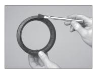
7. LUBRICATE GASKET: Check the gasket to ensure that it is suitable for the intended service. The color code identifies the gasket grade. Lubricate the gasket in accordance with the "Lubricant Compatibility for Gaskets" table above. Always consult the pipe manufacturer for lubricant compatibility requirements.
