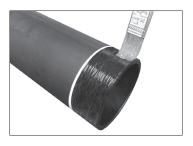
**4. LUBRICATE PIPE END:** Apply a thin coat of lubricant to the pipe end, from the end of the pipe to the paint mark made in step 3.
