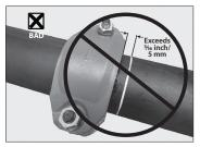
**7. INSPECT BOLT PADS:** Before pressurizing the system, inspect the bolt pads at each joint to ensure that proper assembly is achieved.
