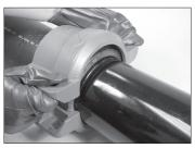
**6. INSTALL HOUSINGS:** Wear gloves while handling coupling housings. The teeth machined into the housings are sharp and can cause injury. Install the housings, ensuring that the teeth are facing toward the HDPE pipe. The key section of the housings must engage into the groove in the steel pipe. Ensure that the gasket remains positioned properly in relation to the groove in the steel pipe and that the mark on the HDPE pipe indicates full insertion into the coupling.
