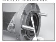
9. LUBRICATE LIP: After the gasket is in place, apply additional lubricant to the outer gasket lip that will seal on the mating flange face. Refer to the "Lubricant Compatibility for Gaskets" table above.
