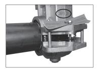
**5a. ASSEMBLE JOINT:** Wear gloves while handling valve. Retainer teeth are sharp and may cause injury. Assemble the joint by inserting the marked HDPE pipe ends into each opening of the valve. Ensure that the flow arrows on the body match system flow direction.
