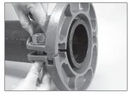
3. INSTALL DRAW BOLTS: Insert the draw bolts into the flange adapter housings. Install a washer onto the end of each bolt. Thread a nut loosely onto the end of each draw bolt.
