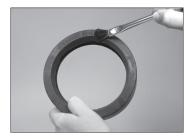
**3. LUBRICATE GASKET:** Check the gasket to ensure that it is suitable for the intended service. The color code identifies the gasket grade. Lubricate the gasket in accordance with the "Lubricant Compatibility for Gaskets" table on page 31. Always consult the pipe manufacturer for lubricant compatibility requirements.
