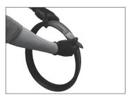
2. LUBRICATE GASKET: Check the gasket to ensure that it is suitable for the intended service. The color code identifies the gasket grade. Lubricate the gasket in accordance with the "Lubricant Compatibility for Gaskets" table on page 37. Always consult the pipe manufacturer for lubricant compatibility requirements.
