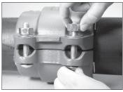
8. INSTALL HARDWARE: Insert the bolts. Install a washer onto the end of each bolt. Thread a nut fingertight onto each bolt. NOTE: Ensure that the oval neck of the bolts seat properly in the bolt holes.
