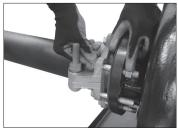
8. INSTALL FLANGE BOLTS AND NUTS: Insert lubricated flange bolts through the flange bolt holes and gasket (when applicable). Join the mating flange with the flange adapter by aligning the bolts with the mating flange holes. Thread nuts finger-tight onto each bolt. NOTE: Flange bolts, nuts, and gasket are not provided.
