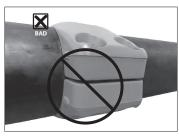
**6. INSPECT BOLT PADS:** Before pressurizing the system, inspect the bolt pads at each joint to verify that proper assembly is achieved in accordance with steps 5a and 5b.
