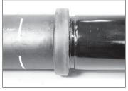
5. ALIGN GASKET: Align and bring the HDPE and steel pipe ends together. Slide the gasket into position by centering it between the mark on the HDPE pipe and the groove in the steel pipe. Ensure that the gasket does not extend into the groove in the steel pipe. NOTE: The space between the pipe ends must never exceed ½ inch/6 mm for 2–4-inch/50–100-mm sizes and ½ inch/8 mm for 5-inch/125-mm and larger sizes.
