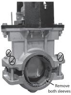
1a. DO NOT DISASSEMBLE THE VALVE: Series 906 Knife Gate Valves are designed so that the installer does not need to remove the assembly hardware for installation. This design facilitates installation by allowing the installer to directly insert HDPE pipe
