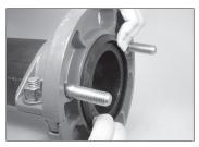
8. INSTALL GASKET: Install the gasket into the cavity between the outside diameter of the pipe and the flange adapter. NOTE: The markings on the outside of the gasket must face the flange adapter. When the gasket is installed correctly, the lettering will not be visible. Ensure that the gasket is completely pressed into this cavity around the entire circumference.
