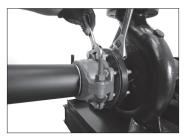
9. TIGHTEN FLANGE NUTS: Tighten all nuts evenly in a crossing pattern, in accordance with a regular flange assembly. Continue to tighten all nuts until the standard, flanged joint torque requirement is reached.
