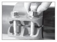
7. INSTALL HARDWARE: Insert the bolts. Install a washer onto the end of each bolt. Thread a nut fingertight onto each bolt. NOTE: Ensure that the oval neck of the bolts seat properly in the bolt holes.
