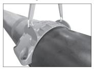
**4b. LIFTING LUGS:** Lifting lugs are provided on IPS couplings (20 inches and larger) and on metric couplings (500 mm and larger) to aid in assembly. Maximum safe lifting lug loads are imprinted on each housing with lifting lugs.
