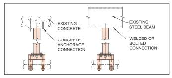
FIGURE 1.2 TYPICAL INSTALLATION OF PRODUCT A81/A82/A83 TO CONCRETE AND STEEL STRUCTURE
