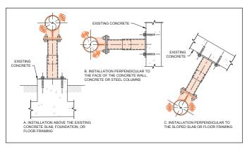
FIGURE 5. ALTERNATE INSTALLATION ORIENTATIONS FOR A81, A82, AND A83 PRODUCTS
