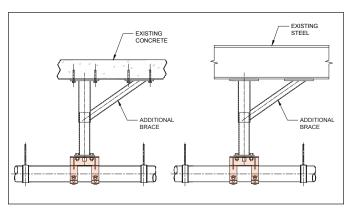
FIGURE 2. TYPICAL INTERMEDIATE STEEL FRAME CONNECTING PRODUCT A84 TO SUPPORTING STRUCTURE
