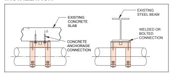
FIGURE 1.1 TYPICAL INSTALLATION OF PRODUCT A84
