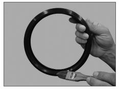
2. CHECK GASKET AND LUBRICATE: Check the gasket to make sure it is suitable for the intended service. The color code identifies the gasket grade. Apply a thin coat of Victaulic Lubricant or silicone lubricant to the gasket sealing lips and exterior.
