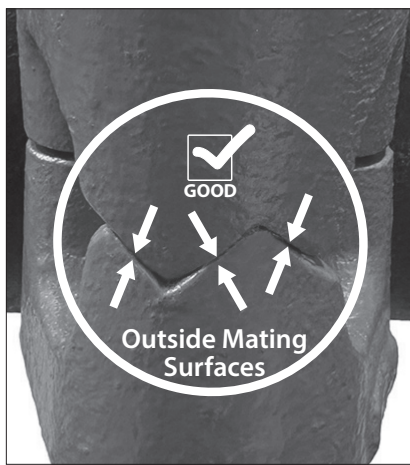
PROPERLY ASSEMBLED JOINT – METAL-TO-METAL CONTACT AS INDICATED AT ALL OUTSIDE MATING SURFACES
