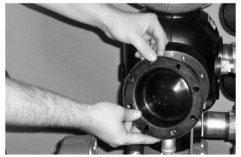
3. Remove the diaphragm from the valve body.
