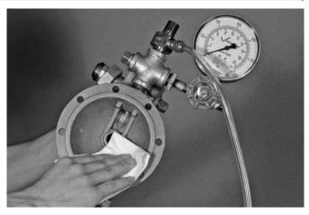
Clean the inside of the diaphragm cover to remove any foreign material.
